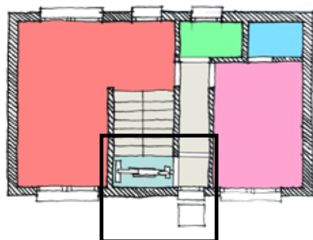
Windbreak (double door) and storage under the stairs
